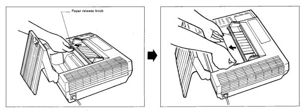
3. Unwrap the roll of recording paper and load it as shown in the figures on the inside of the cover.
